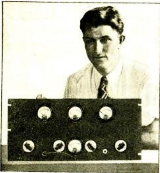
Front view of the 35-Watt Exciter Unit. The cost of building the unit can be reduced by eliminating some of the meters but, if possible, they should all be used.
