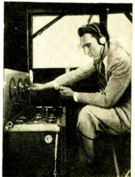
▲ A "field-strength" measuring set installed in the Laboratories' Fairchild plane.
