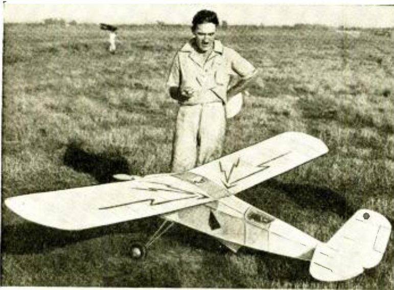
The radio-controlled plane on the ground preparatory to take-off. Note the control switch in the operator's hand.
